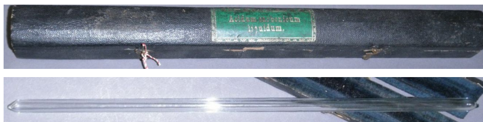
Figure 3. (Colour online) Natterer tube with \text{CO}_2 used in lectures to show critical opalescence. © Collection in the Observatory of the Monastery Chremsminster.
