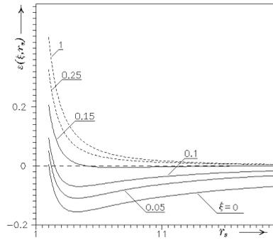
Figure 5. Dependence of the total energy of the generalized model on the parameter  $\xi$ . The calculations are based on (2.8), (2.9), (3.1), (3.4).
