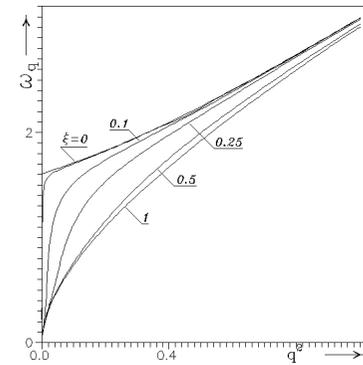
Figure 8. Dependence of the spectrum of the collective excitations  $\omega_q$  on the parameter  $\xi$  at the fixed value of  $r_s = 5.0$ . ( $\xi$  has the values 0.0; 0.05; 0.1; 0.25; 0.5; 1.0). The calculations are based on (4.2), (4.12).
