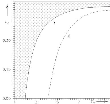
Figure 6. Stability and existence region of the generalized model as a function of the parameters  $r_s$  and  $\xi$  at  $A = 1$ . Curve 1 is the solution of (3.6), curve 2 is the solution of (3.7).
