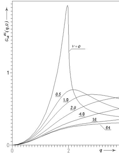
Figure 1. Dynamic local-field correction function of the electron liquid model ( $\xi \rightarrow 0$ ,  $A = 1$ ,  $G_{id}^{EL}(q; \nu)$  (2.2) at  $r_s \rightarrow 0$ .
