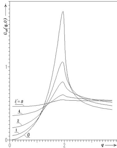
Figure 2. Static local-field correction function  $G_{id}(q; 0)$  (2.2) in dependence on the parameter  $\xi^*$ .
