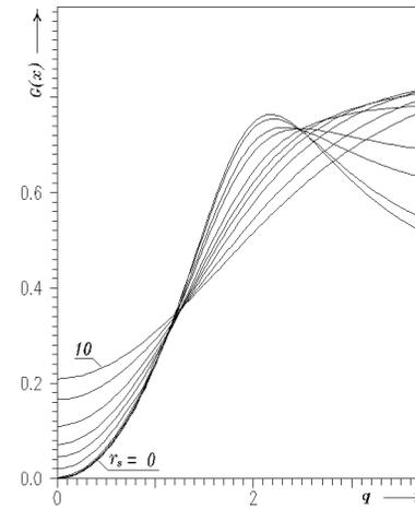
Figure 4. Dynamic local-field correction function  $G(x)$  in dependence on the parameter  $r_s$  in the approximation (2.8), (2.9) ( $r_s$  has the values 0.0; 0.1; 0.5; 1.0; 2.0; 3.0; 4.0; 5.0; 7.0; 10.0) at  $A = 1.0$ ,  $\xi = 0.25$ ,  $u = 1.0$ .
